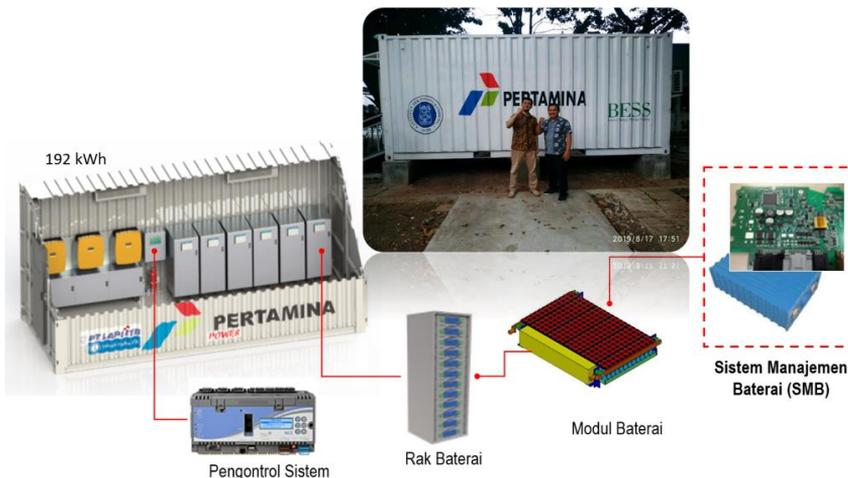
**Gambar 2.8** Sistem SBPE berukuran kontainer
