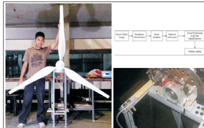
Gambar 17 Set Up model tes hasil rancangan & torque dynamometer
