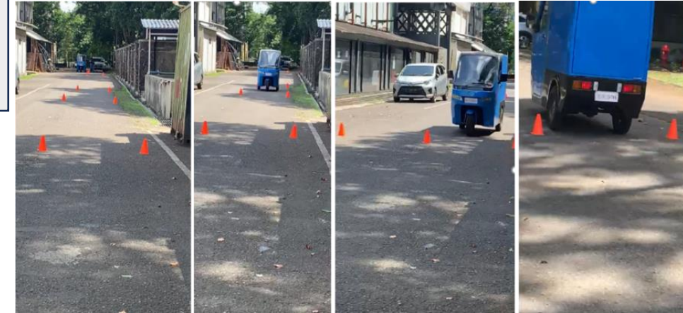
Double Lane Change (ISO 3888-1:2020) v = 21 \text{ km/h}
