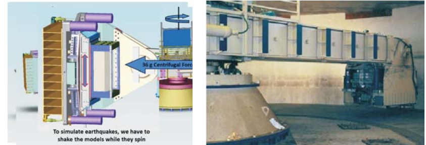
Gambar 31. Alat Centrifuge di University of California Davis-USA (Sitar, 2016)
