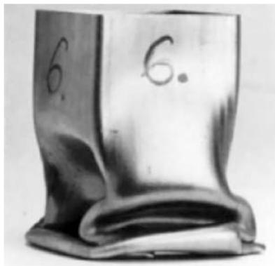
**Gambar 3.1** *Asymmetric Folding Mix Mode A* [23] [8]
