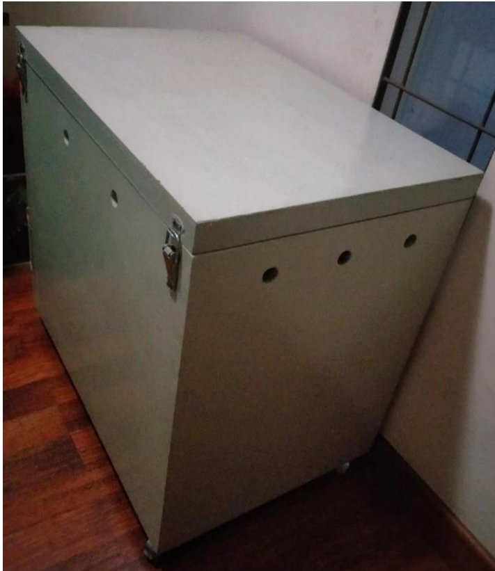
Gambar 36 Model Masa Termal Internal berisi PCM
