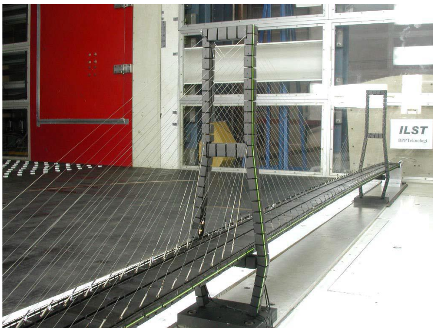
Gambar 16 Model penuh jembatan Suramadu di seksi uji Indonesian Low Speed Wind Tunnel (ILST) (Fariduzzaman, et al., 2004)
