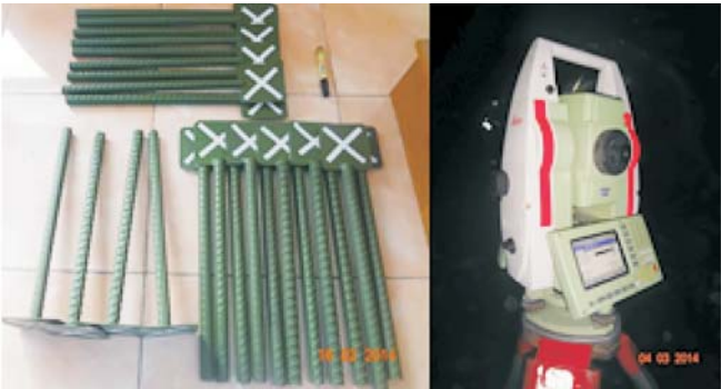
Gambar 4.20 Pin (target) dan total station
