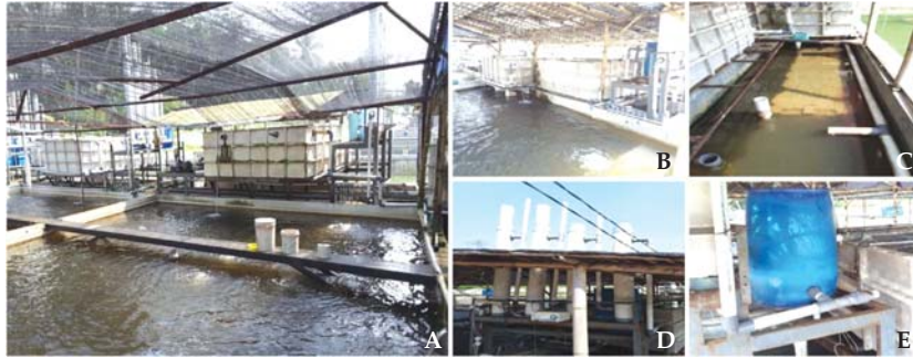
Gambar 10. (A) Penerapan sistem RAS di industri perikanan budidaya air tawar di Cianjur; (B) tanki kultur; (C) settling tank; (D) protein skimmer; (E) carbon active tank.
